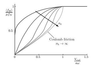
Figure 1: Effective friction-velocity characteristics for longitudinal excitation
