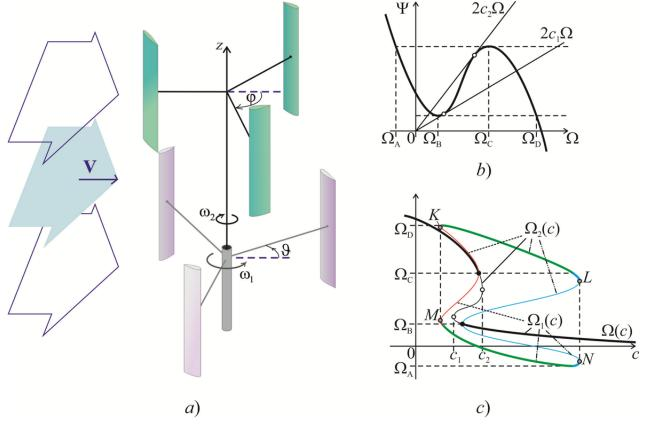
Fig. 1 *a*) The scheme of the double Darrieus wind turbine; *b*) The qualitative view of  $\Psi(\Omega)$ ; *c*) The qualitative bifurcation diagram. The following conditions are sufficient for asymptotical stability of a fixed point of (2):
