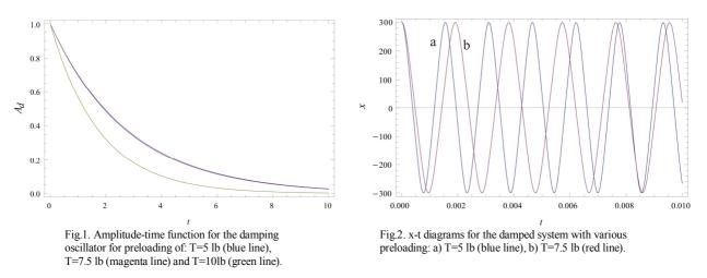
In Fig.2 the solution of equation (2) for various preloading force is plotted. It can be concluded that the period of vibration is higher for larger preloading. Even for small change of the preloading force the frequency of vibration is shorten significantly.
