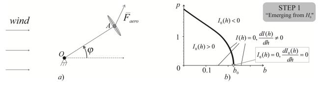
Fig. 1 a) An aerodynamic pendulum (top view); b) Bifurcation diagram of periodic trajectories emerging from trajectories of H<sub>0</sub>.
