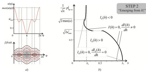
Fig. 2 a) On a phase portrait of the system  $H_1$ ; b) Bifurcation diagram of periodic trajectories emerging from trajectories of  $H_1$ .
