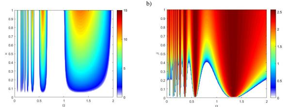
Fig1. Influence of vibration regeneration mechanism expressed by  $\alpha$  ( $\beta$ =0.1) a), and friction effect expressed by  $\beta$  ( $\alpha$ =0.1) on stability of non-trivial solution (the colors indicate the value of vibrations amplitude).
