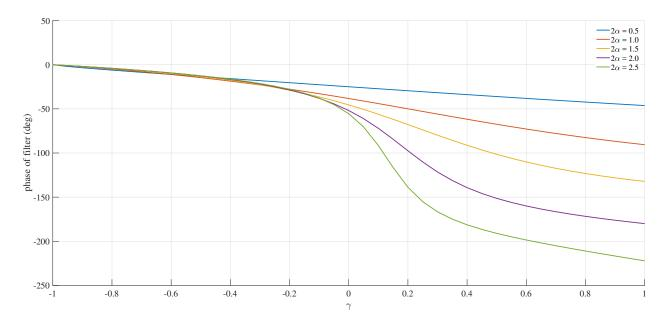
Figure 3: Variation of phase lag in degrees vs  $\gamma$  for different values of  $\alpha$
