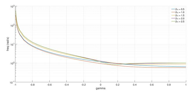
Figure 4: Shift of corner frequency with change in  $\gamma$  for different values of  $\alpha$
