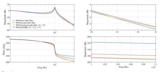
Figure 6: Open loop frequency response for all controller configurations provided. On the left is the overall open loop frequency response. On the right top is zoom in at the bandwidth and on the right bottom is at high frequencies where noise attenuation is necessary
