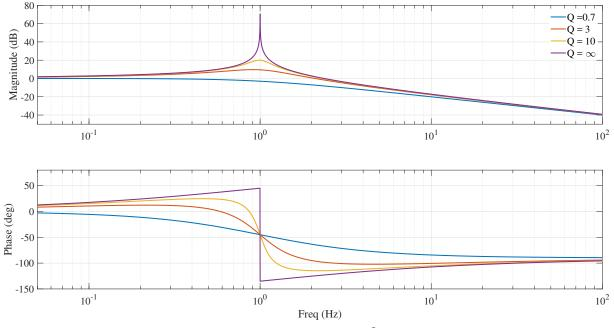
Figure 1: Bode plots of first order filter realized using  $H^{2\alpha}(s)$  for different Q-factors
