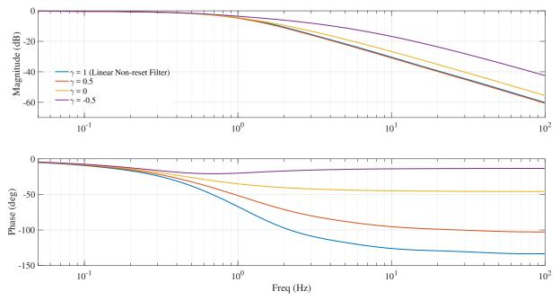
Figure 2: Bode plots of GFrORE obtained using describing function for order  $2\alpha = 1.5$  for different values of  $\gamma$
