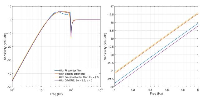
Figure 8: Sensitivity plots for all controller configurations with zoom-in provided at low frequencies
