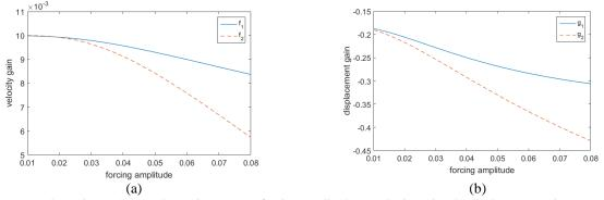
Figure 3. Level dependent gains at every forcing amplitude (a) velocity gains (b) displacement gains
