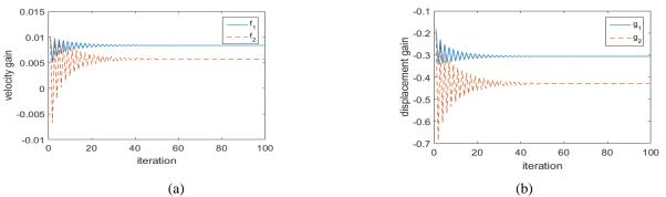
Figure 1. The feedback control gains at every iteration (a) velocity gains (b) displacement gains
