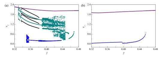
Figure 3: Bifurcation diagrams for the capsule system constructed for varying mass ratio  $\gamma$ , (a) without control ( $k_p = 0$ ) and (b) with control ( $k_p = -0.2$ ), calculated for  $\beta = 3$ ,  $\xi = 0.05$ ,  $\delta = 0.02$ ,  $\alpha = 1.6$ ,  $\omega = 1.1$ , and  $v_s = 0.1$ .
