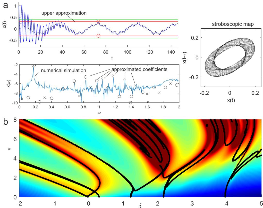
Figure 1: a) time signal of a numerical simulation of the frequency modulated delayed Mathieu equation with quasi-periodic excitation, its stroboscopic map and the corresponding spectrum b) Colormap denotes the maximal position, the black lines denote the corresponding stability boundary
