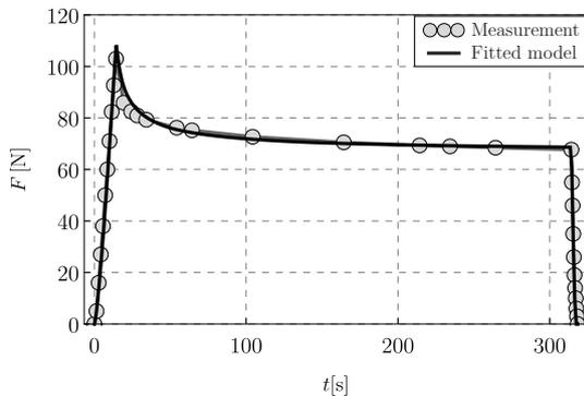
Figure 4: Comparison of the  $F(t) - t$  curves of the fitted model and the experimental results of the pellet
