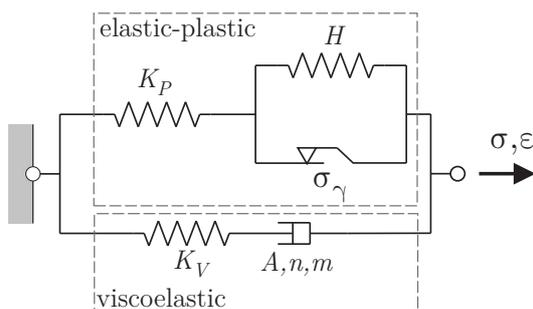
Figure 2: The one-dimensional representation of the two-layer viscoplastic model
