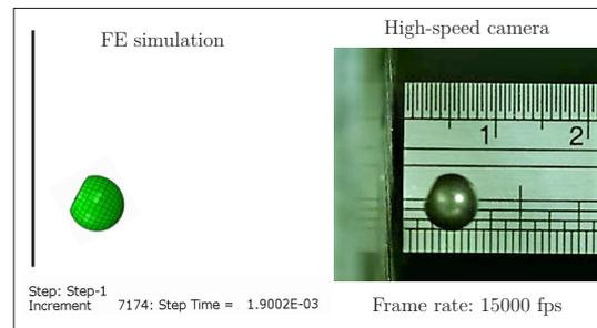
Figure 5: Comparison of the deformed shape of the pellet after the impact to rigid wall in case of FE simulation and high-speed camera measurement with input velocity  $v = 36$  m/s
