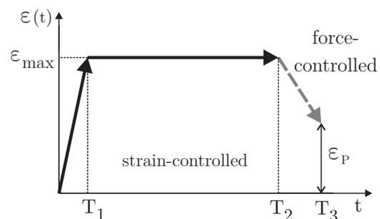
Figure 3: The load input of the uniaxial cyclic relaxation test applied in the parameter-fitting process
