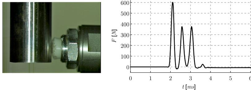
Figure 1: The phenomena of multiple-hitting during the hammer excitation of a dummy tool
