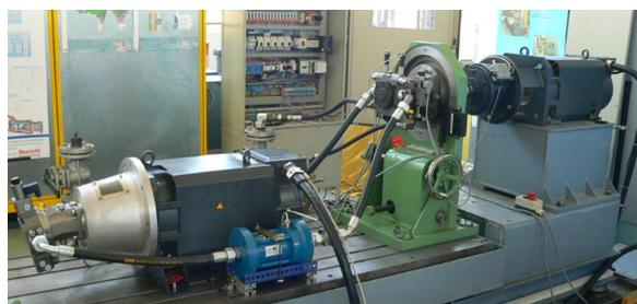
(a) Drive train with a closed-circuit hydrostatic transmission.
