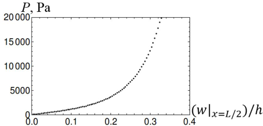
Figure 1. Static pressure-deflection curve. The abscissa shows central deflection.
