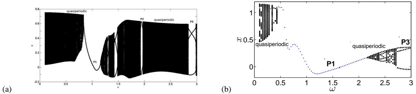
Figure 2: Bifurcation diagram with  $\omega$  as the parameter (a)  $f_0 = 0.1$  (b)  $f_0 = 0.5$
