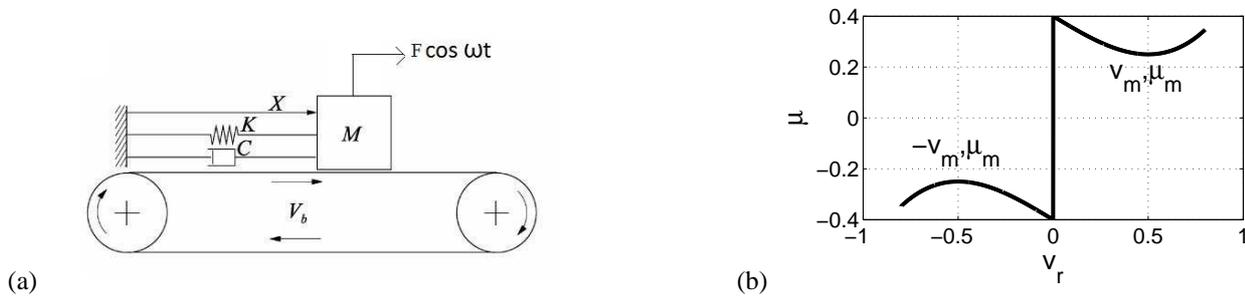
Figure 1: (a) Model of a discontinuous oscillator (b) Stribeck friction model
