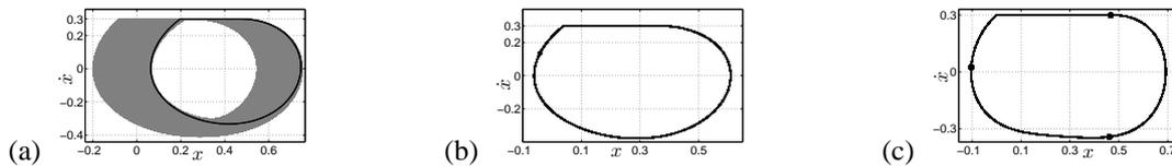
Figure 3: (a) Quasiperiodic solution for  $\omega = 0.34$  (b) P1 solution for  $\omega = 0.97$  (c) P3 solution for  $\omega = 2.9$ .
