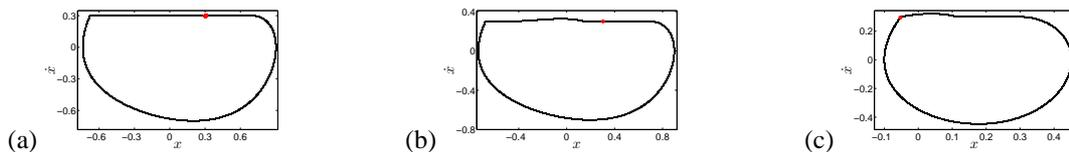
Figure 4: Phase plane plots (a) stick-slip  $\omega = 0.65$  (b) adding sliding  $\omega = 0.66$  (c) switching sliding  $\omega = 1.5$
