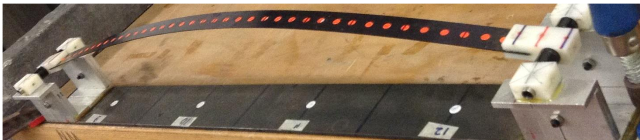
Figure 1 The elastic beam model (Dynamics-Acoustics & Diagnostics Laboratory, NTUA) used as a physical model to predict nonlinear dynamics phenomena-with interesting energy flow properties-in flexible beams with multiple equilibrium states. The experimental dynamics are three-dimensional with strong nonlinear cross-coupling.
