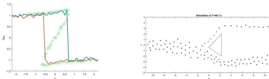
Figure 2: Left: stable and unstable branches of steady states with green crosses, obtained by the state observer method. Right: the pedestrian motion for an unstable steady state at  $(f, \mu) = (-0.46, -0.6995)$ .
