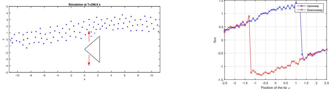
Figure 1: Left: Snapshot of the pedestrian flow. Right: Hysteresis behaviour of the instantaneous measure flux  $f$ .
