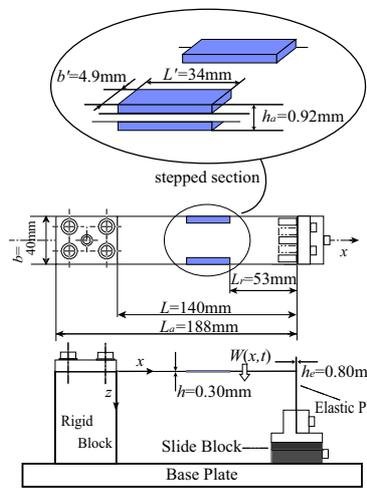
Fig.1 Beam and fixture
