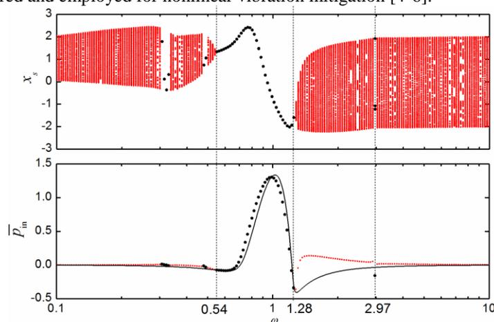
Figure 2. Power flow characteristics of the forced Van der pol oscillator. (a) Bifurcation diagram and (b) time-averaged input power ( $\alpha = 0.5, f = 1$ ). Black dots: periodic responses; red dots: quasi-periodic responses. Lines: analytical approximations.
