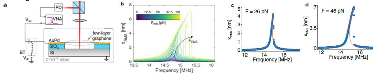
Fig. 1. (a) The schematic experimental set up; (b) experimentally measured non-linear amplitude-frequency response curves; (c) comparison between the experimental (dots) and identified curve (red line) for  $F=26pN$ ; (d) comparison between the experimental (dots) and identified curve (red line) for  $F=46pN$ .
