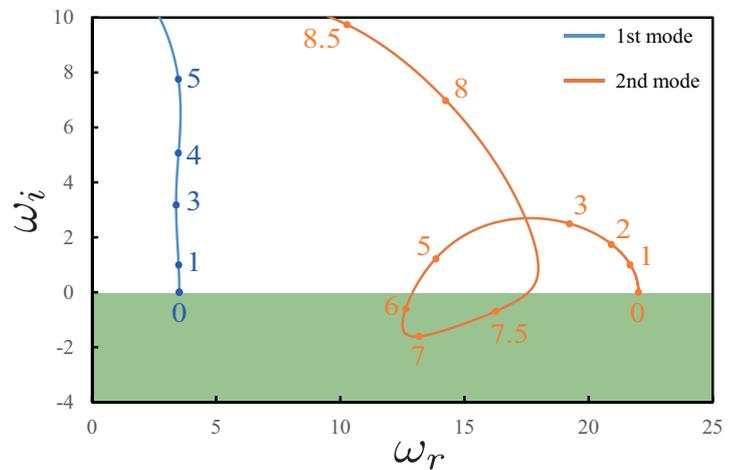
Figure 2: The complex frequency of the two lowest modes of the cantilevered pipe as a function of the dimensionless flow velocity,  $U$  ( $\beta = 0.232, \gamma = 0$ )
