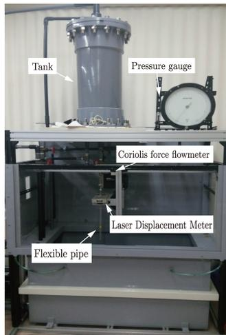
Figure 3: Experiment Apparatus
