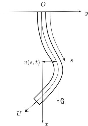
Figure 1: Analytical model of fluid-conveying pipe
