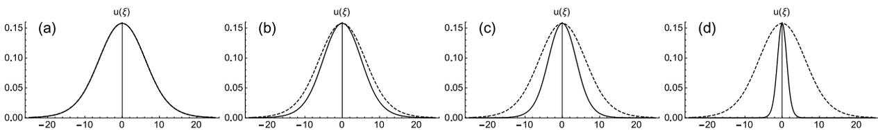
Figure 1: The effect of the second dispersive term  $H_2 U_{XXTT}$  on the width of a solitary wave. Here  $P = -10$ ,  $Q = 40$ ,  $H_1 = 2$ ; (a)  $H_2 = 0$ , (b)  $H_2 = 2$ , (c)  $H_2 = 4$  and (d)  $H_2 = 6$ . Dashed line with  $H_2 = 0$  is plotted for reference.
