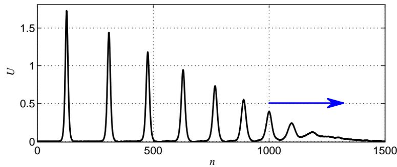
Figure 2: Formation of soliton train propagating from left to right with smaller amplitude solitons traveling faster than the larger amplitude ones. Here  $P = -0.2186$ ,  $Q = 0.004230$ ,  $H_1 = 72.14$ ,  $H_2 = 1.000$ , dimensionless time  $t \approx 9800$ .
