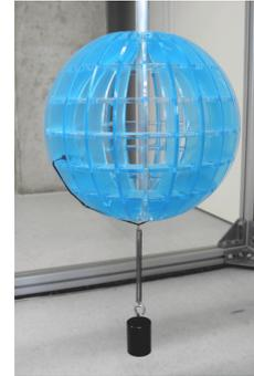
Figure 7: Sphere of the pendulum with an additional mass connected to the sphere by a spring.
