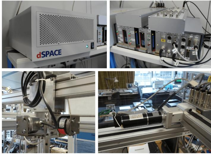
Figure 2: dSPACE autobox (top left), servo amplifiers (top right), Cardan joint and encoders (bottom left), DC motor (bottom right).
