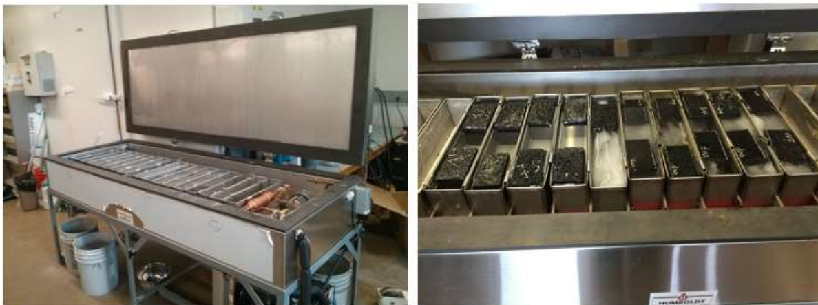
Figure 1: F-T cycle testing set up using an ASTM C666 apparatus (left) and specimens after a number of F-T cycles (right)
