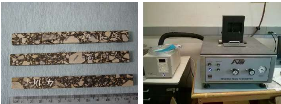
Figure 1: F-T cycle testing set up using an ASTM C666 apparatus (left) and specimens after a number of F-T cycles (right)
